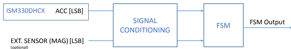
Figure 2. State machine in the ISM330DHCX
