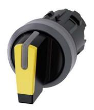
Selector switch, illuminable, 22 mm, round, plastic with metal front ring, yellow, selector switch, short, 3 switch positions I-O-II, latching, actuating angle 2x45°, 10:30h/12h/13:30h, with laser labeling, inscription or symbol Customer-specific selection with SIRIUS ACT configurator (CIN)
