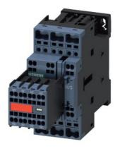
Power contactor, AC-3 38 A, 18.5 kW / 400 V 2 NO + 2 NC, 230 V AC 50/60 Hz, 3-pole Size S0, Spring type terminal Captive auxiliary switch
