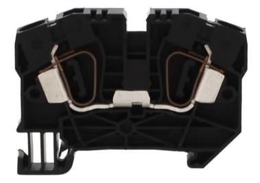
Feed-through terminal, Tension-spring connection, Mounting type: Mounting rail TS 35/7.5, Rated cross-section: 6 mm<sup>2</sup>, Width: 8.1 mm, Colour: Black
