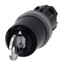
Key-operated switch IKON, 22 mm, round, plastic with metal front ring, lock number 360012K1, with 2 keys, 3 switch positions I>O<II, momentary contact type, actuating angle  $2x45^{\circ}$ , 10:30h/12h/13:30h, key removal O, Z=50-unit packaging
