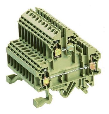
Double-level terminal/block variant, Screw connection, Mounting type:Mounting rail TS 35/7.5 and TS 32, Rated cross-section: 2.5 mm<sup>2</sup>, Colour: Beige
