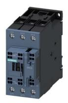
traction contactor, AC-3 51 A, 22 kW / 400 V 1 NO + 1 NC 24 V DC, 0.7-1.25\* US, with varistor, 3-pole, size S2, spring-loaded terminal
