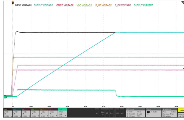
Figure 28. Startup by ON/PD (no load)
