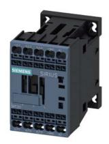
power contactor, AC-3 12 A, 5.5 kW / 400 V 1 NO, 220 V AC, 50 Hz 240 V, 60 Hz, 3-pole Size S00, Spring-type terminal
