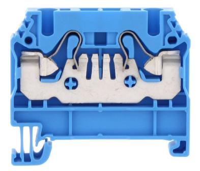
Feed-through terminal, Push-in connection, Mounting type: Mounting rail TS 35/7.5, Rated cross-section: 4 mm<sup>2</sup>, Width: 6.1 mm, Colour: Blue
