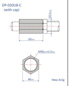
Note: When attaching, make sure that the side without a bearing chamfer is the impact surface.
