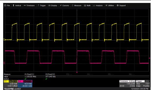
Figure 6-10. Fsw = 577 kHz with external sync = 1.155 MHz (577 kHz x 2 = 1.154 MHz)
