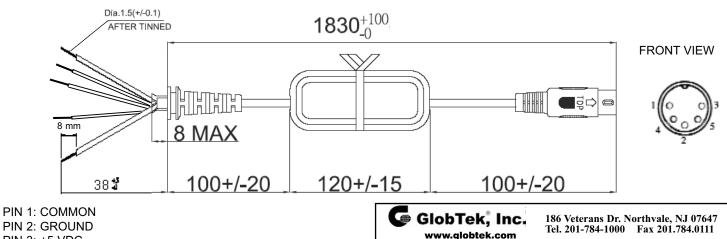
PIN 2: GROUND PIN 3: +5 VDC PIN 4: -12 VDC PIN 5: +12 VDC SHELL: N/C
