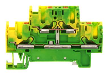
Protective-earth double-level terminal, Push-in connection, Mounting type: Mounting rail TS 35/7.5, Rated cross-section: 2.5 mm², Width: 5.1 mm, Colour: Green-yellow
