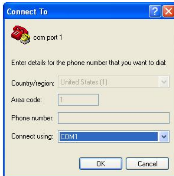
Figure 4 Choose correct COM port
