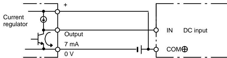
NPN open-collector output
