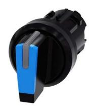
Selector switch, illuminable, 22 mm, round, plastic, blue, selector switch, short, 3 switch positions I>O<II, momentary contact on the left, latching on the right, actuating angle  $2x45^{\circ}$ , 10:30h/12h/13:30h
