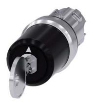
key-operated switch Siemens, 22 mm, round, metal, shiny, lock number SSG10, with 2 keys, 3 switch positions I-O-II, latching, actuating angle  $2x45^{\circ},\,10:30h/12h/13:30h,$  key removal I+O+II, with laser labeling, upper case and lower case, always upper case at beginning of line
