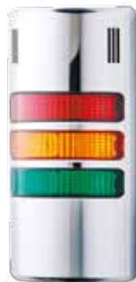
Order number: HD90-Q91 Colours: red/orange/green Function: LED steady beacon, buzzer steady or pulsing tone Housing colour: chrome Nominal voltage: 230-240 V AC
