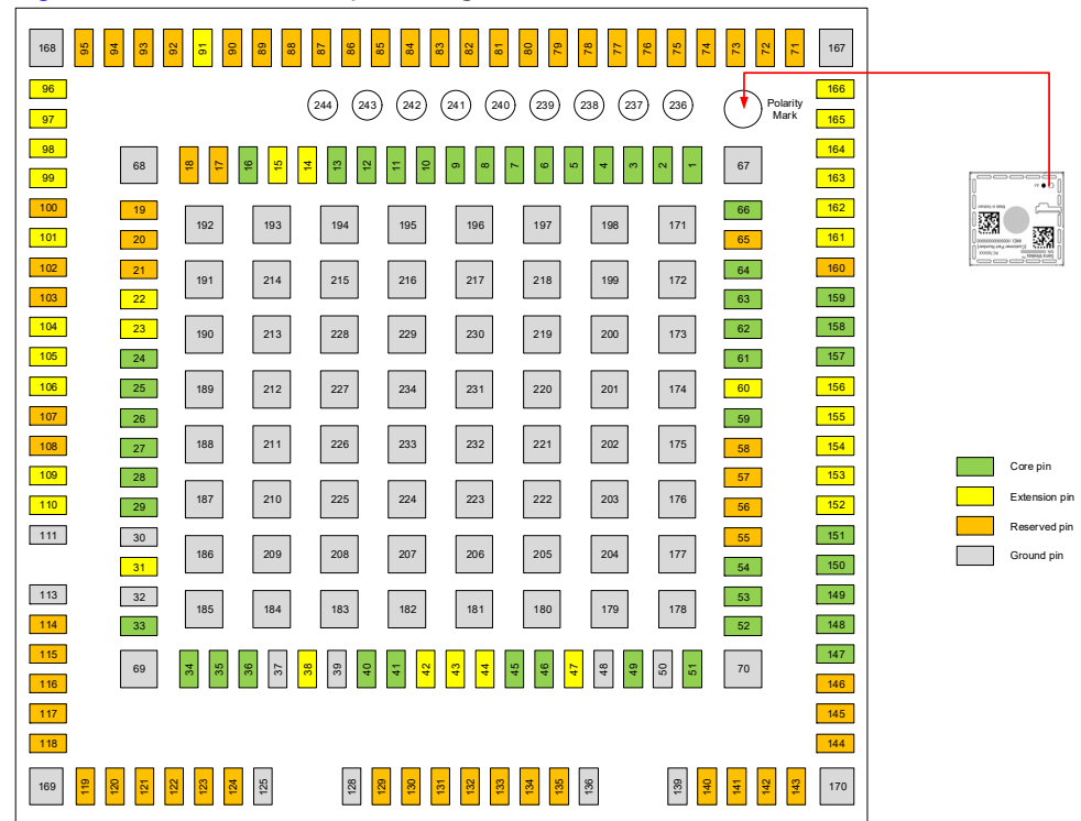
Figure 10-1: Pin Configuration (Top View, Through Module)
