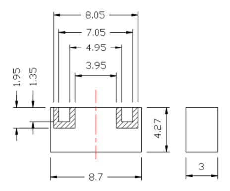
Dimensions in mm Tolerance : ±0.25
