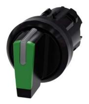
Selector switch, illuminable, 22 mm, round, plastic, green, selector switch, short, 3 switch positions I-O<II, left latching, right momentary contact type, actuating angle  $2x45^{\circ}$ , 10:30h/12h/13:30h Z=50-unit packaging
