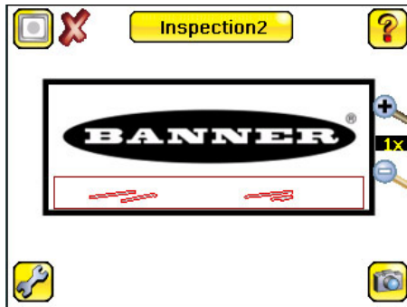
Figure 111. Blemishes Found During the Inspection
