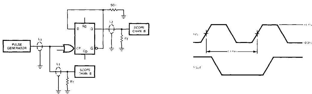
$L_1$  and  $L_2$  = equal length  $50\Omega$  impedance lines
