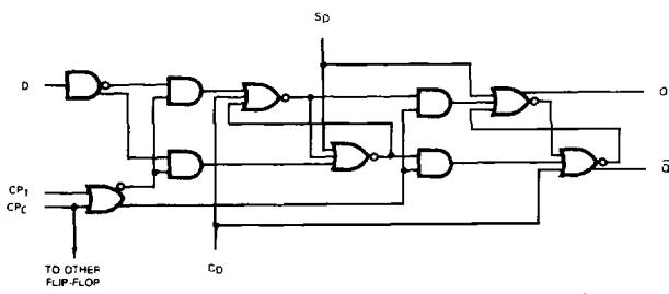
Note that this diagram is provided for understanding of logic operation only. It should not be used for evaluation of propagation delays, as many gate functions are achieved internally without incurring a full gate delay.
