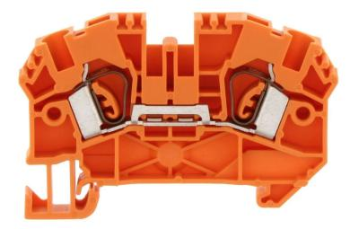
Feed-through terminal, Tension-spring connection, Mounting type: Mounting rail TS 35/7.5, Rated cross-section: 4 mm<sup>2</sup>, Width: 6.1 mm, Colour: Orange
