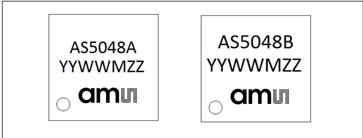
Figure 39: Package Markings for AS5048A & AS5048B
