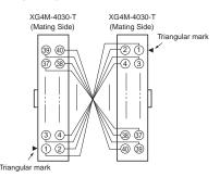
Note: Wire the pins 1:1 so that the Connector pin numbers match.
