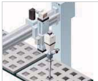
Confirming suction of electronic component
