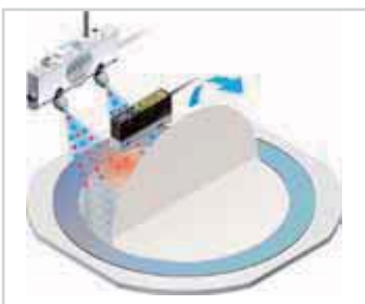
Measuring surface potential when removing BG sheets
