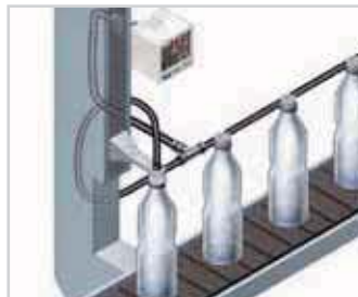
Air-leak test for PET bottles
